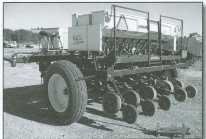
Figure 2 - This Rough Rider drill manufactured by the Truax Co. incorporates some of the newest advances in rangeland drill technology.
