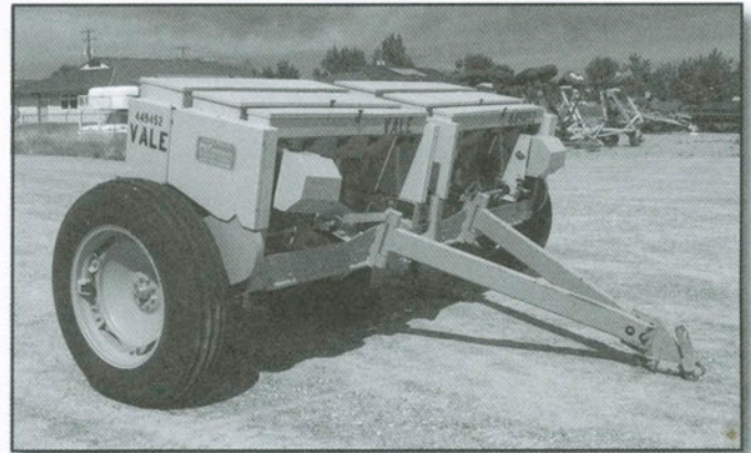
Figure 1—The basic design and function of the rangeland drill has changed little over the last 50 years.
