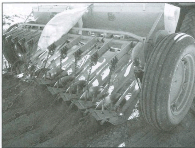
Figure 3 Heavy curved disks clear vegetation and create furrows for the dropped seed. Weight can be added to each disk arm.
